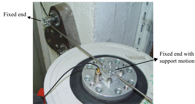
Fig. 6. Both fixed ends for measurement of the vibrations of the cable.
